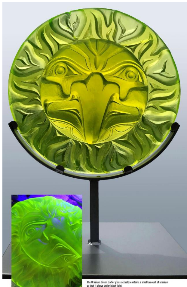
The Uranium Green Gaffer glass actually contains a small amount of uranium so that it glows under black light.
